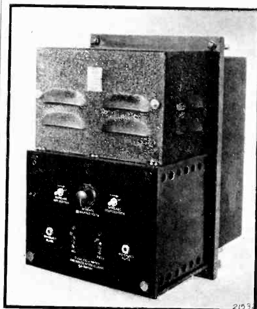
Compact electronic regulator operating on less than one microwatt of control energy
